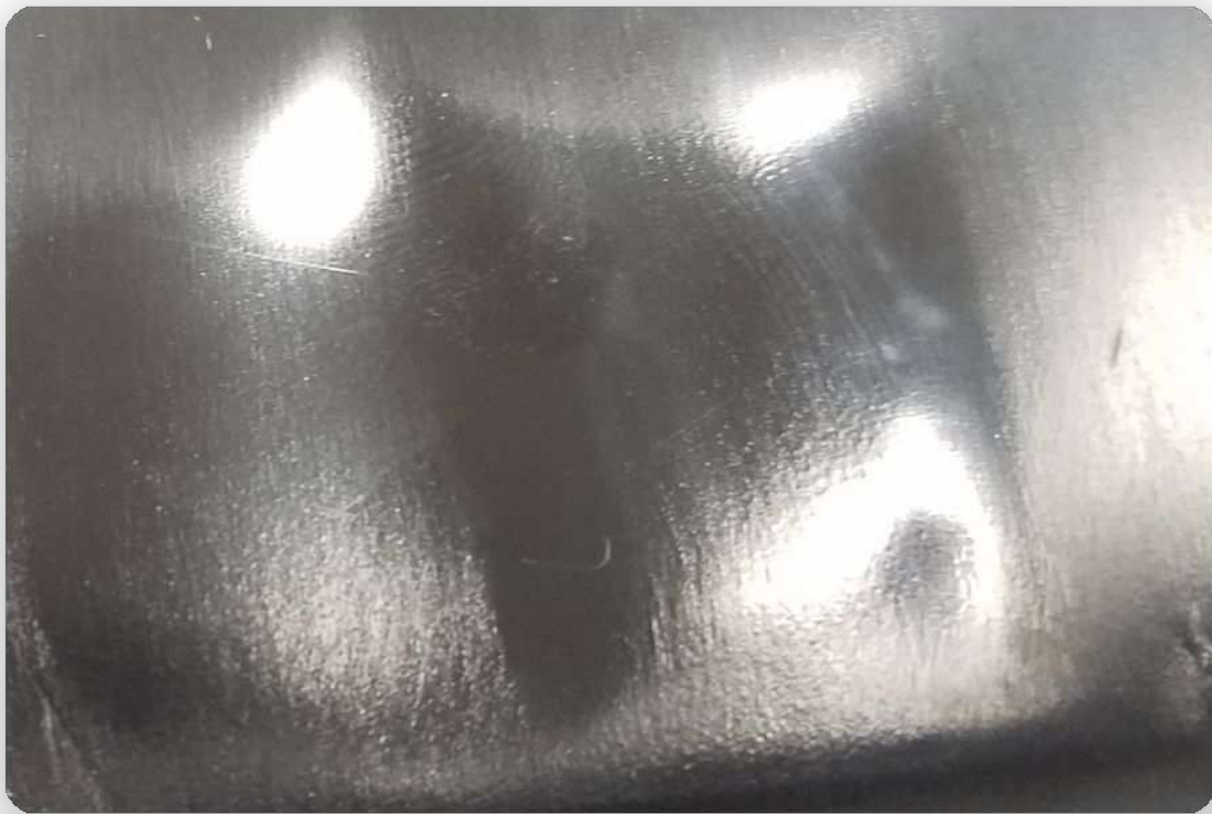
An example of a part with sink mark
