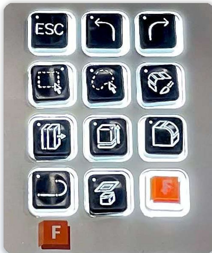
The finished overmolded keycaps complete with engraving
